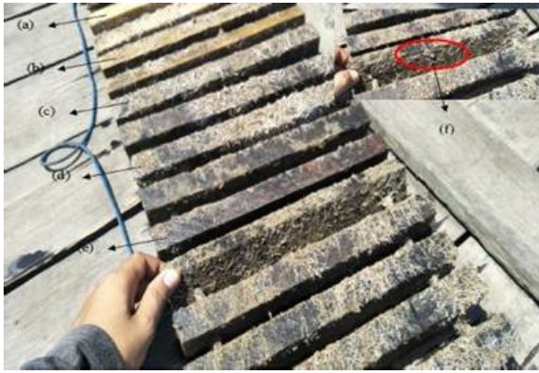
Fig. 5. Samples condition after two months bioassay (a) A. falcataria (b) V. cofassus (c) Diospyros sp. (d) D. indica (e) C. inophyllum , (f) Shells that stick to the samples
